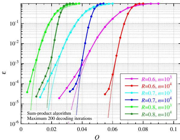
**Fig. 3** Simulated block error rates  $\varepsilon$  of LDPC codes of length  $n = 10^3$  and  $n = 10^4$  and code rates  $R = 0.6$ ,  $R = 0.7$  and  $R = 0.8$  as a function of quantum bit error rate  $Q$
