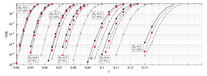
Fig. 3. FER over the BSC with crossover a probability  $\varepsilon$  for several LDPC codes with coding rates  $R_0 = 0.3$ ,  $R_0 = 0.4$ ,  $R_0 = 0.5$  and  $R_0 = 0.6$ , and two different proportions of punctured symbols,  $\pi = 5\%$  and  $\pi = 10\%$ .
