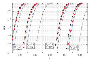
Fig. 2. FER over the BEC with crossover probability  $\varepsilon$  for different intentional puncturing strategies. Two LDPC codes with coding rates  $R_0=0.5$  and  $R_0=0.6$ , and two different proportions of punctured symbols,  $\pi=5\%$  and  $\pi=10\%$  were used. See inset in Fig. 1 for symbols and line-styles.
