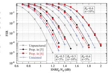
Fig. 1. FER over the AWGN as a function of the signal-to-noise ratio (SNR). Two LDPC codes with coding rates  $R_0=0.5$  and  $R_0=0.6$ , and two different proportions of punctured symbols,  $\pi=5\%$  and  $\pi=10\%$  were used.
