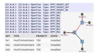
Fig. 9. Three captures showing the OpenFlow domain working: OpenFlow local messages, the installed intents via SSH, and the ONOS GUI with the intents drawn on top.
