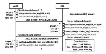
Fig. 3. Diffie-Hellman and QKD key exchange protocol integration.
