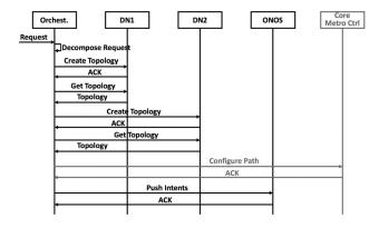
Fig. 5. Distributed virtual infrastructure deployment and configuration workflow.
