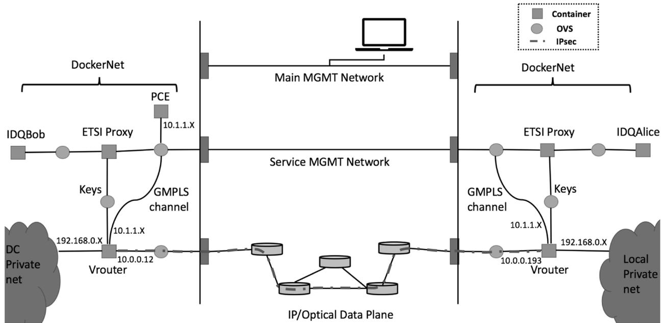
Fig. 6. Logical scheme describing the network used for the end-to-end quantum encryption service via IPsec. The left part shows the DC management and data networks, with a QKD domain (Bob) and a virtual router connected to a PCE. The right part exposes the local network, connecting the other virtual router to the remote PCE and the other QKD domain (Alice). The intermediate area exposes the packet/optical network.
