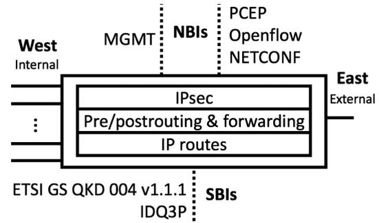
Fig. 1. Schematic view of the virtual router capabilities and interfaces.
